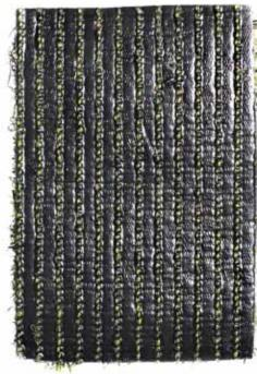
Samples of artificial grass are available so you can decide on the right weight and color for your yard or courtyard. The underside of the swatch shows how the blades of grass are sewn on the plastic backing. Holes are perforated to allow water to drain through the artificial turf into the soil.
